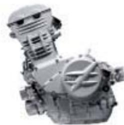
The F800 models are the first to feature the all-new 798-cc **parallel twin**, which is sure to excite riders with its balanced performance characteristics and impressive power output.
