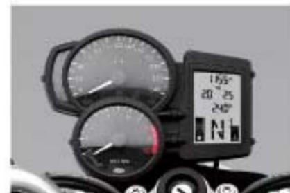
**TPC** (Tyre Pressure Control) continuously monitors tyre pressure, and alerts the rider to any abnormalities via the display and/or a warning light.
