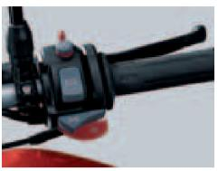
The heated grips can be adjusted to two levels and ensure warm hands even in extreme weather.
