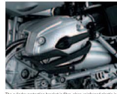
The cylinder protection bracket in fibre-glass-reinforced plastic is mainly designed for use on the road, protecting the cylinder head cover from damage.
