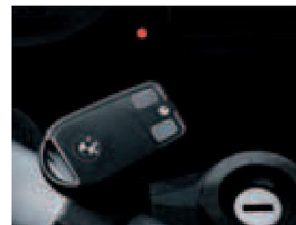
The anti-theft warning system reacts to every change in position with a clearly audible warning signal and flashing light.\*
