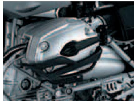
The cylinder protection bracket in fibre-glass-reinforced plastic is mainly designed for use on the road, protecting the cylinder head cover from damage.
