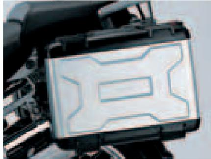
The waterproof vario pannier features a patented adjustment mechanism. The volume can be reduced from a total of 68 litres (29 litres left, 39 litres right) to 50 litres (20 litres left, 30 litres right). This is particularly advantageous in city traffic, since this reduces the width by 120 mm.
