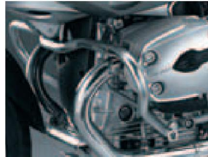
The robust engine protection bracket with its stable steel tube construction offers protection from damage in the cylinder area on rough terrain.
