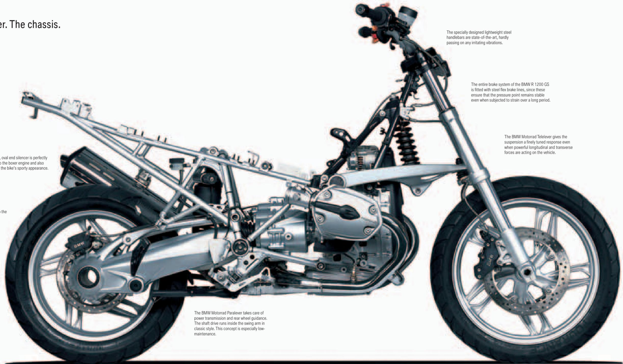
The specially designed lightweight steel handlebars are state-of-the-art, hardly passing on any irritating vibrations.
