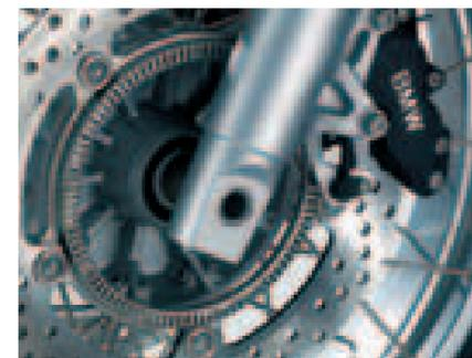
Safety guaranteed: BMW Motorrad Integral ABS, in the partially integral version for sports-style riding. Can be deactivated for off-road use.
