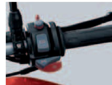
The heated grips can be adjusted to two levels and ensure warm hands even in extreme weather.
