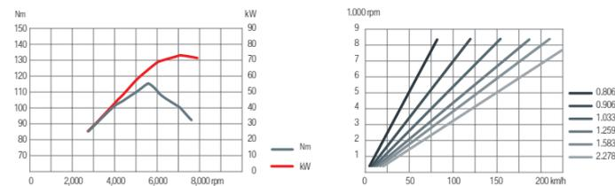
Power and responsiveness: an output of 74 kW (100 bhp) at 7,000 rpm, and a maximum torque of 115 Nm at 5,500 rpm.
